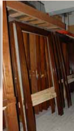
Above, two doors in the finish shop. Disassembled pieces are kept together during the refishing process. Then the doors and trim are labeled with room numbers and stored, right, to await reinstallation after each phase of the project is completed.
