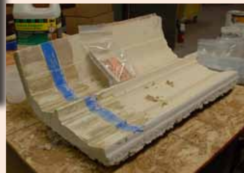
Above, crown molding in the south center corridor was hidden by dropped ceiling for years. Right, a removed section of the molding allows staff to conduct paint analysis and plan for repair and restoration of this detail.
