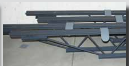
Below center, the rugs will be rolled on large PVC pipes which will more uniformly bear the weight of the rug and minimize stretching. Left and right, the tubes will be placed on bar joists fitted with curved brackets to support and stabilize the weight as the rugs are handled. As used during Capitol construction to move the heavy marble columns, a chain hoist and simple physics will help move the heavy rugs up and into place.
