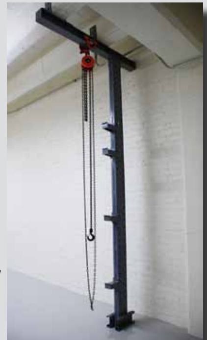
Above, one rug has been placed in temporary storage in the newly completed space. This rug rests on saw horses and a small metal pipe, the previous method of storage, which put stress on the rug. Right, each support frame is bolted to the floor and ceiling for stability. The rugs to be stored may weigh up to 1000 pounds. For ease of placement and access, preservation architects devised a special trolley system to raise and lower the bar joists into place on the brackets.
