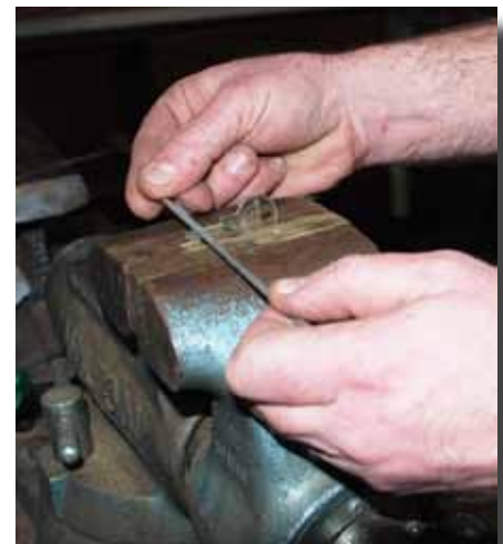
Above, OCC staff creates a new desk key from blank key stock. The slow careful filing process restored the desk drawer locks to working condition.
