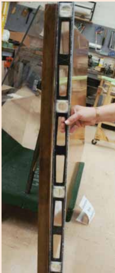
Above, shop staff holds a level to the desk top revealing a quarter inch bow in the wood.
