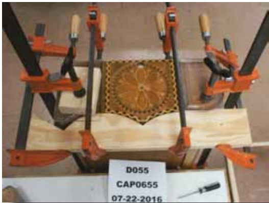
Above and below, OCC staff created custom jigs and blocks to allow precise gluing and clamping as they repaired the many damaged areas of the desk drawers. They added blocks to the drawer rails, inset right, to stop the drawers and prevent future damage, documenting the non-original additions.
