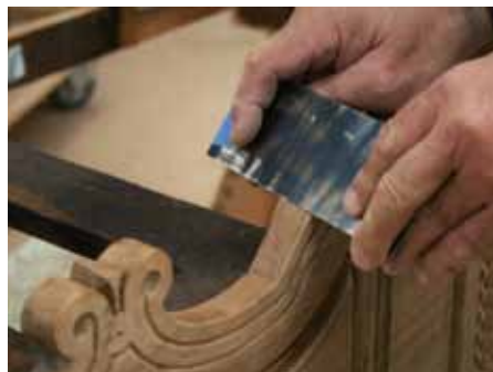
The craftsmen creating the Italian Renaissance desks which inspired the design of the Nebraska Governor's Desk would have used scrapers in their finish work, just as, left, Capitol staff did during this project.
