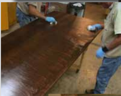
An important step reinforced the structure of the desk. Above left, the missing drawer skirts were recreated and above right, a frame was added to support the desk top and prevent future sagging. Top and bottom left, the application of dark walnut stain was one of the final steps in the project.
