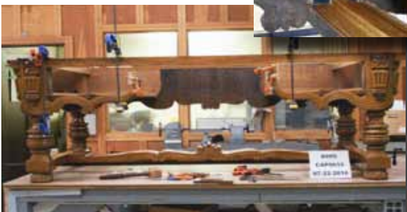
Above and below, OCC staff created custom jigs and blocks to allow precise gluing and clamping as they repaired the many damaged areas of the desk drawers. They added blocks to the drawer rails, inset right, to stop the drawers and prevent future damage, documenting the non-original additions.
