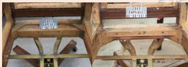
Above, the chair's seat supports had been altered, but not in a consistent manner. Some of the modifications impacted the function of the chair legs and material removal had weakened the frame supports.
