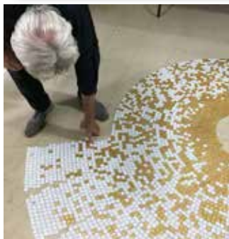
Left, tile designer, Doug Harris at the Bisazza studio in Florida created the pattern in small panels, allowing gaps in the outer edge to accommodate the bowl’s curve. The bowls were stripped to bare bronze to provide maximum adherence. Simulated weather testing revealed the commonly available grouts used for tile were too rigid; expansion and contraction caused the glass tile to crack. Above, a flexible adhesive, similar to that used to hold tiles on the space shuttles is applied to the bowl. Above right, each panel of tile had a brightly colored placement number attached so they could be laid according to the pattern.
