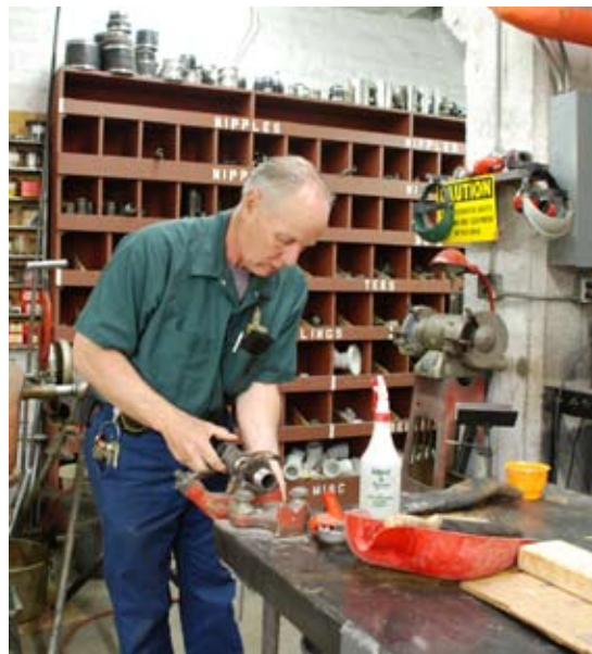
Jerry Allen, Office of the Capitol Commission Maintenance staff plumber rebuilds a section of pipe before returning it to service.
