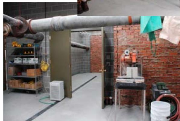
A wet cutting room was created, above, to contain dust and debris from large scale projects. Note the newly installed yellow air line for pneumatic tools beside the wet room door. Tools and equipment are now organized and stored within easy reach of the main work area.
